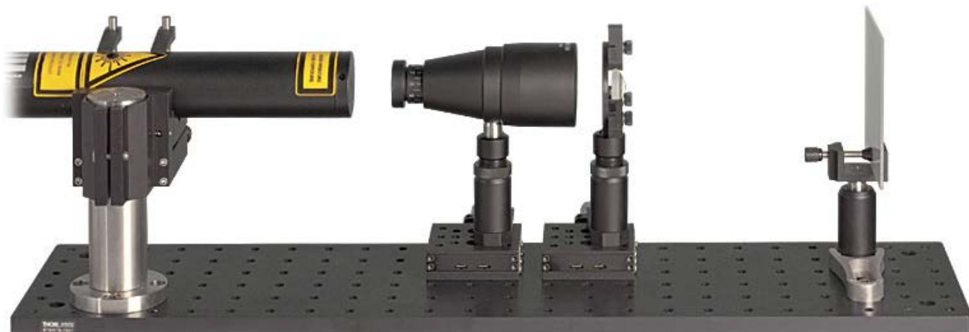
Fig 2: A setup including a HeNe laser, beam expander, axicon, and diffuser.
